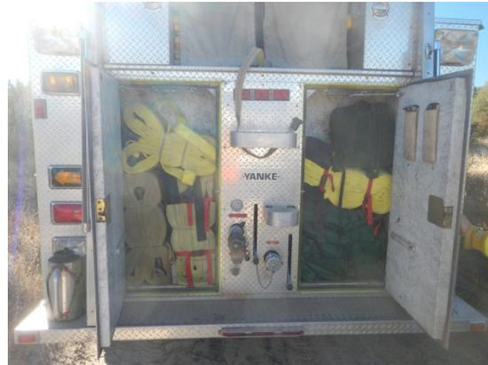
**Photo 4:** ECMs observed Type III Fire Engines equipped with 1,200-foot hose extensions.
