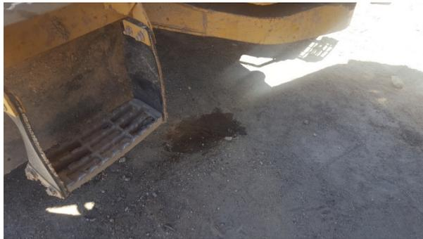
**Photo 3:** ECMs observed stained soil under construction equipment at site G-12.
