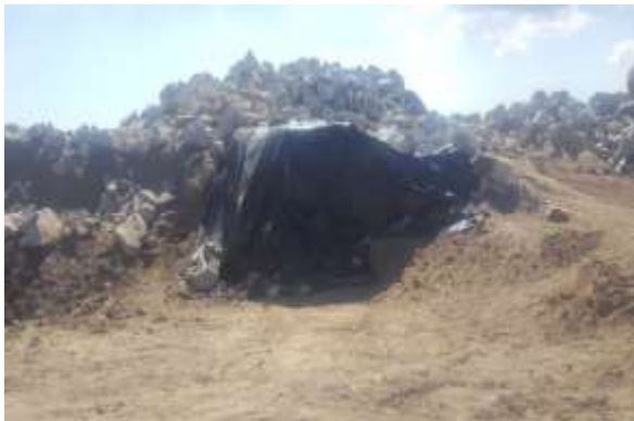
Photo 3: ECMs observed a cover over a stained boulder to keep any runoff from spilling onto the ground in accordance with the Spill Prevention Control and Countermeasure Plan. Tule Wind LLC is anticipated to apply a cleaner/degreaser to clean the boulder.
